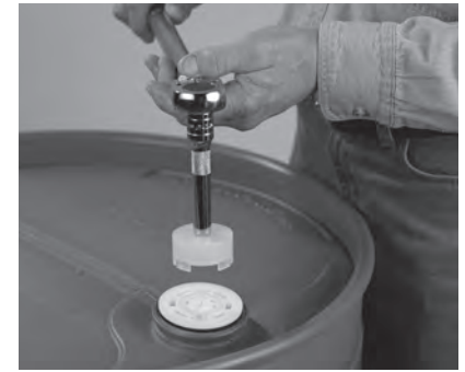
3. Torque insert with drum wrench or 1/2" drive torque wrench and a Colder torque socket tool. (Colder PN 2290301). Note: Torque to 25 ft-lb (34 N-m).
