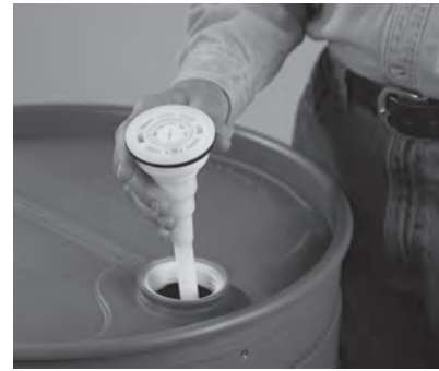
2. Place the drum insert assembly in drum.
