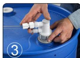
Example of safer chemical dispensing through a closed system:
