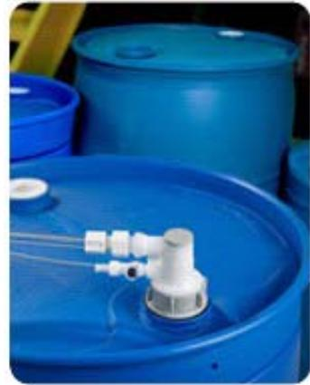
Another popular dispensing method is a semi-closed system that pumps the liquid out of a drum or container. In these systems, a dip-tube draws chemicals from vertically-oriented containers using an attachable hand or electric pump. While a step in the right direction, the semi-closed dispensing system requires a dip-tube that needs to be removed and re-inserted each time a new drum is used, exposing the end user to drips, leaks and fumes during transfer.
